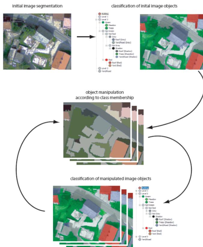
**Figure 2.** GEOBIA principles: Iterative process of knowledge-based image segmentation and classification (from: Hofmann et al. 2008)
