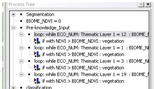
Figure 3: Branching/ Looping algorithm in CNL translating biomes into variables holding NDVI thresholds which are automatically used in the image analysis.
