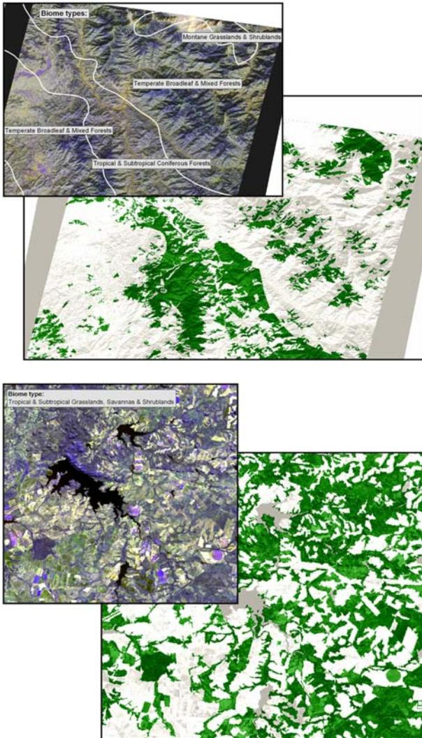
Figure 4: Classification of vegetated areas in Kashmir (upper image) and Zimbabwe (below). For both images the same rule set is used – changes concerning NDVI thresholds are automatically performed by reading biome type information from a georeferenced map (upper left and upper right).
